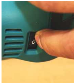
▲ Speeds are adjusted using the dial at the rear of the saw
